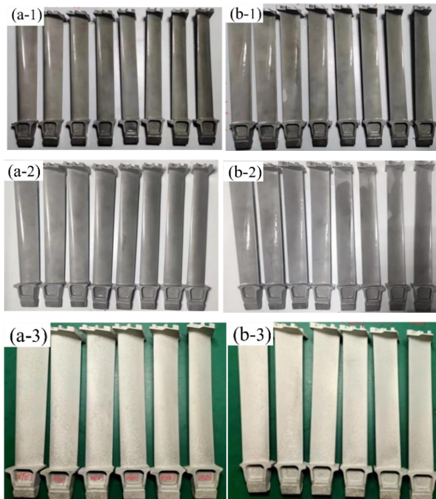
Fig. 1. Surface grain size of blades after corrosion at three types of shell preheating temperature: a – convex; b – concave; (1)1110 °C; 2 – 1150 °C; 3 – 1180 °C
